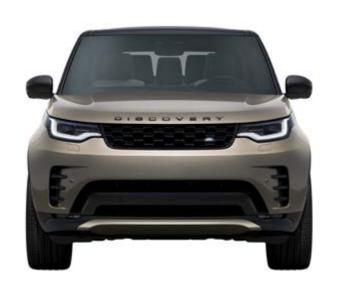
Width 2,073mm mirrors folded Width 2,220mm mirrors out
